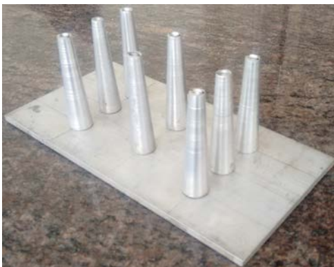
Figure 6. Solid pin fins with staggered arrangement.
