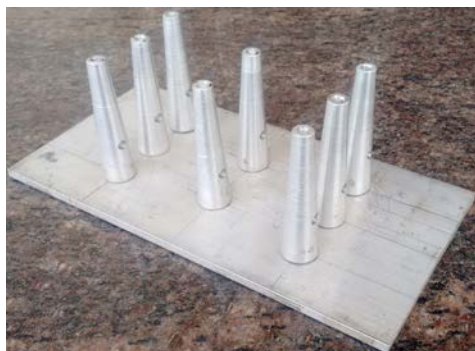
Figure 7. Perforated pin fins with staggered arrangement.
