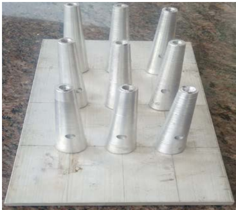
Figure 5. Perforated pin fins with inline arrangement.
