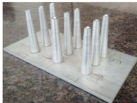
Figure 4. Solid pin fins with inline arrangement.
