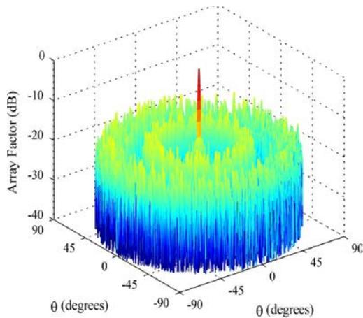
Fig.15: Normalized array factor for the optimized polyfractal array with 319 elements.
