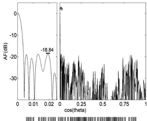
Fig.5: 256 element genetically optimized polyfractal with its radiation pattern
