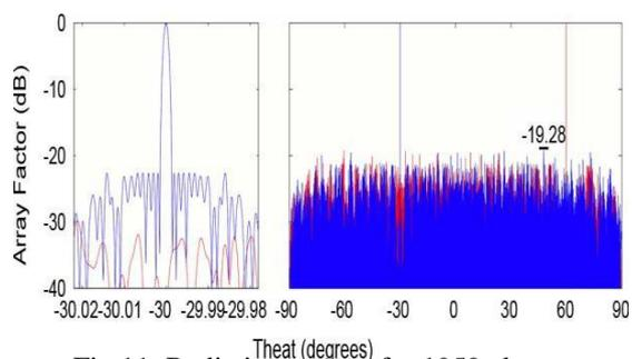
Fig.11: Radiation pattern for 1959 elements optimized polyfractal array.
