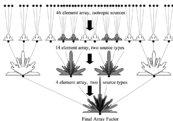
Fig.2: Rapid recursive beamforming algorithm for a two generator polyfractal array.
