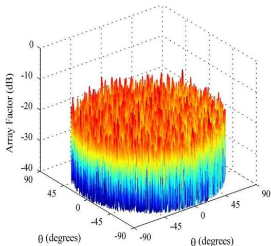
Fig.16: The corrupted radiation pattern for a micro-UAV swarm based on the 319 element optimized polyfractal array.
