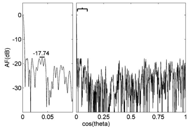
Fig.4: 178 element genetically optimized polyfractal with its radiation pattern.
