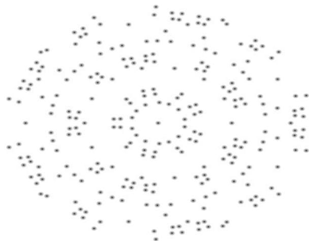
Fig.14: 319 elements of polyfractal array effected by Gaussian noise  $\sigma=0.1\lambda$ .
