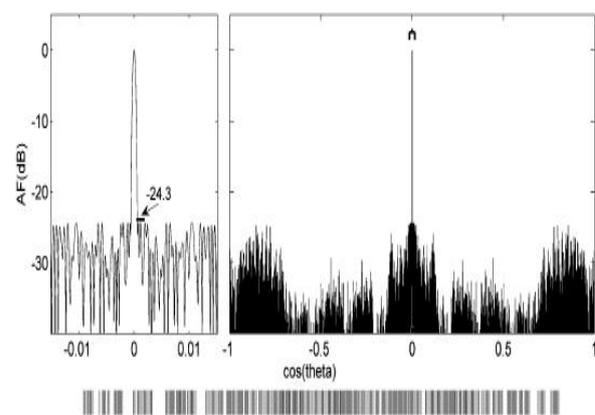
Fig.9:1616 element optimized polyfractal array using generator- autopolyplidity process and its radiation pattern.
