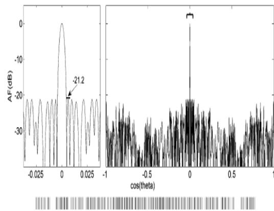
Fig.7: 256 element optimized polyfractal array using generator- autopolyplidity process and its radiation pattern.
