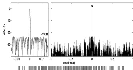
Fig.8:1406 element optimized polyfractal array using generator- autopolyplidity process and its radiation pattern.
