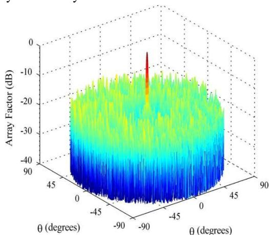
Fig.17: The phase corrected radiation pattern for a micro-UAV swarm based on the 319 element optimized polyfractal array.
