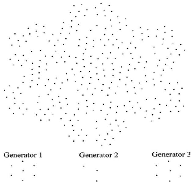
Fig.13: Construction of planer 319 elements optimized polyfractal array using 3 generators.
