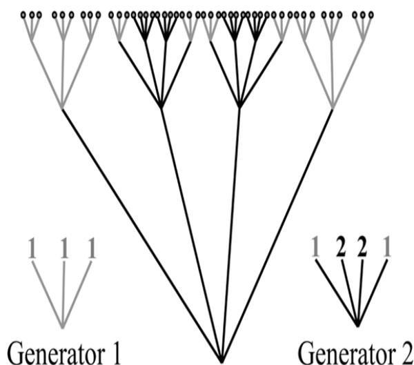
Fig.1: Construction of a 46-element polyfractal array using connection factors.
