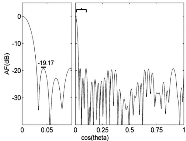
Fig.3: 46 element genetically optimized polyfractal with its radiation pattern
