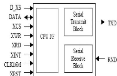
Figure 2: UART Block Diagram
