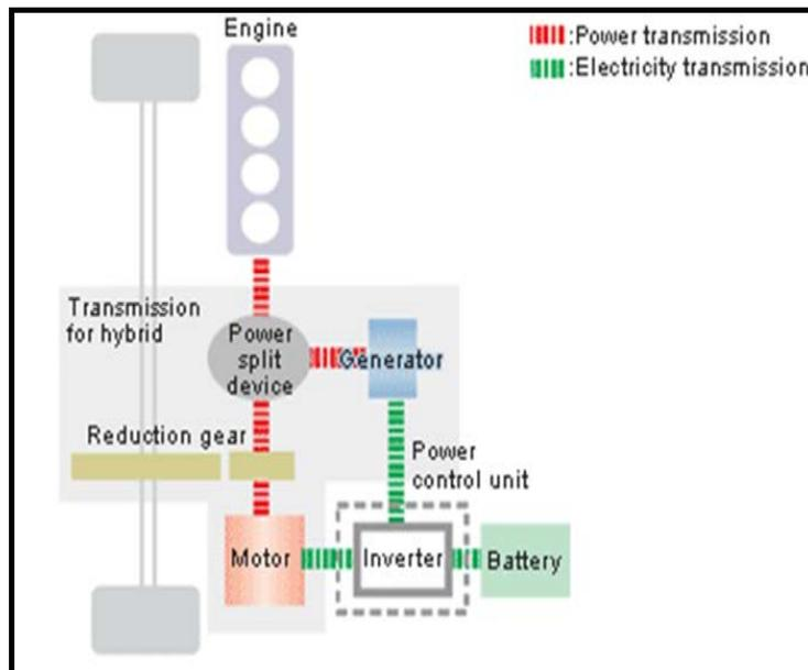
**Fig 7:Power flow through a Series-parallel hybrid**
