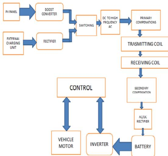
Fig1: A block diagram for modular charging unit
