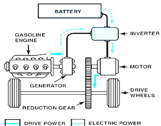
Fig5: Power flow through a series hybrid.
