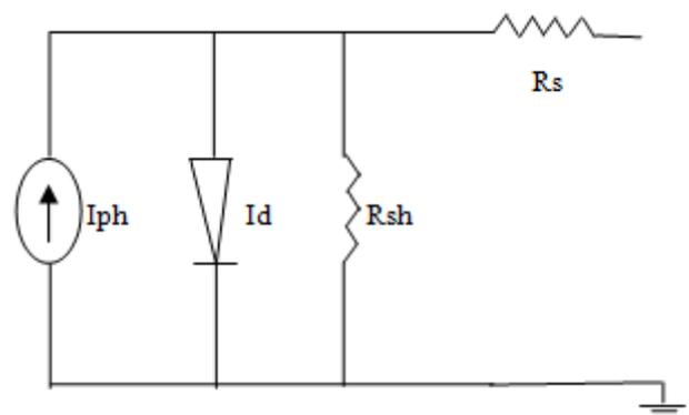
Fig3 :solar diode model of pv
