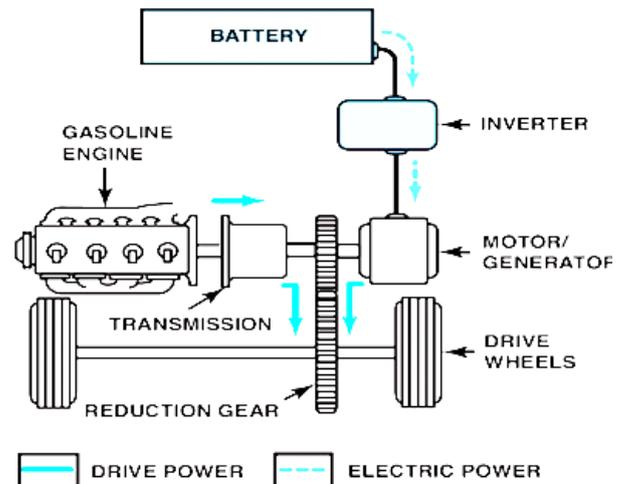
**Fig6: Power Flow through A Parallel Hybrid**
