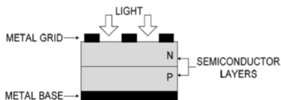
Fig2:Solar pv cell
