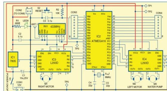
**Fig. 2- Receiver Module**
