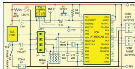
**Fig. 3- Transmitter Module**
