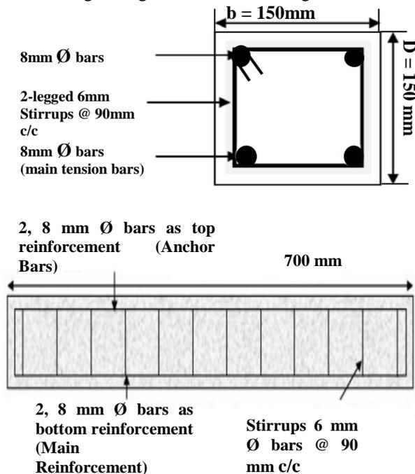
Figure 1. Reinforcement details of beam
