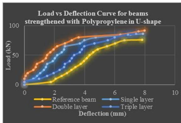
**Graph 1. Load vs Deflection curve for beams strengthened with polypropylene fabric**
