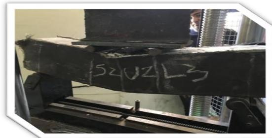
Figure 6. Crushing and debonding of triple layer of polyester fabric from concrete
