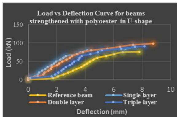
**Graph 2. Load vs Deflection curve for beams strengthened with polyester fabric**
