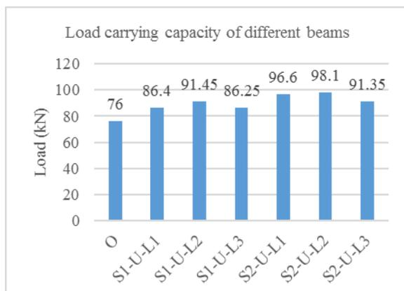
**Graph 4. Load carrying capacity of different beams**
