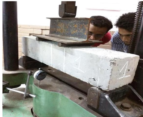
Figure 2. Beam testing set-up
