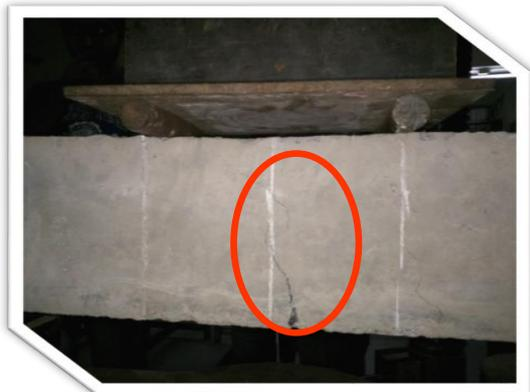
Figure 3. Flexural failure of reference beam
