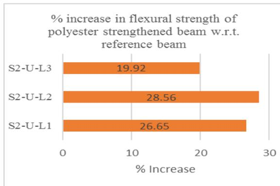
**Graph 4. Comparison of change in flexural strength of beams strengthened with polyester compared with reference beam**
