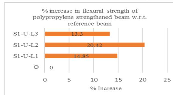
Graph 3. Comparison of %change in flexural strength of polypropylene strengthened beam w.r.t reference beam
