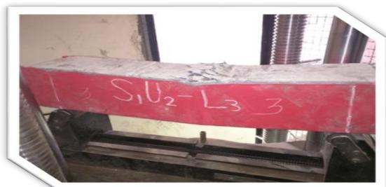
Figure 4. Crushing of concrete in compression and debonding of polypropylene fabric of triple layer
