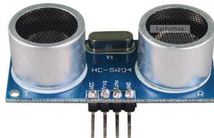
**Figure 4.6 Ultrasonic sensor**
