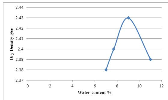
**Fig. 6 Compaction Curve for 30% Crusher Dust**
