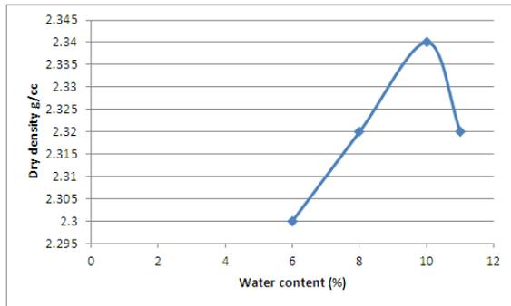
**Fig. 2 Compaction Curve for 10% Crusher Dust**
