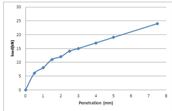
**Fig. 5 CBR Test Curve for 20% Crusher Dust**
