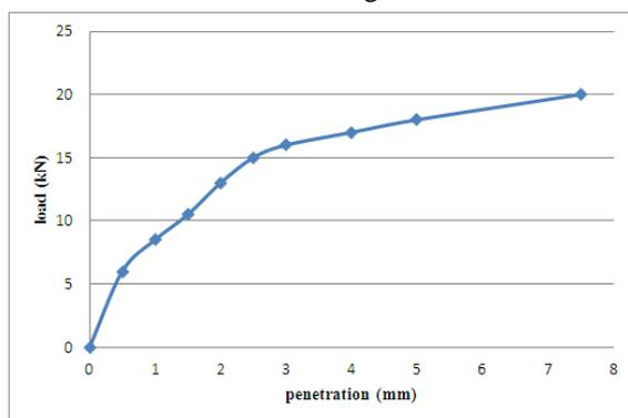
**Fig. 3 CBR Test Curve for 10% Crusher Dust**
