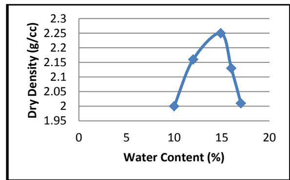
**Fig. 10 Compaction Curve for Field Soil**
