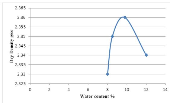
**Fig. 4 Compaction Curve for 20% Crusher Dust**
