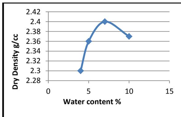
**Fig. 8 Compaction curve for 40% crusher dust**
