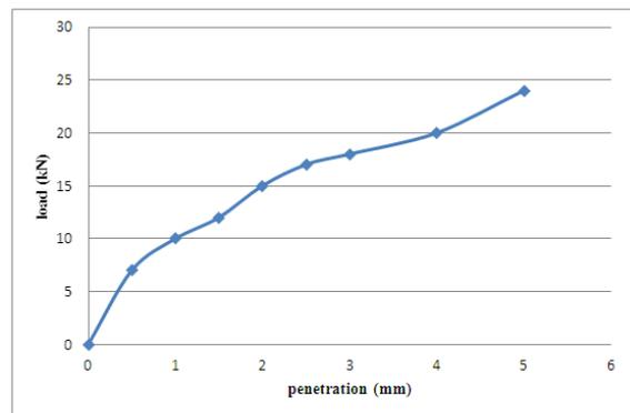
**Fig. 7 CBR Test Curve for 30% Crusher Dust**
