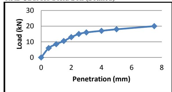
**Fig. 11 CBR Test for Field Soil**
