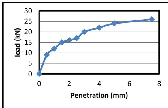
**Fig. 9 CBR Test Curve for 40% Crusher Dust**
