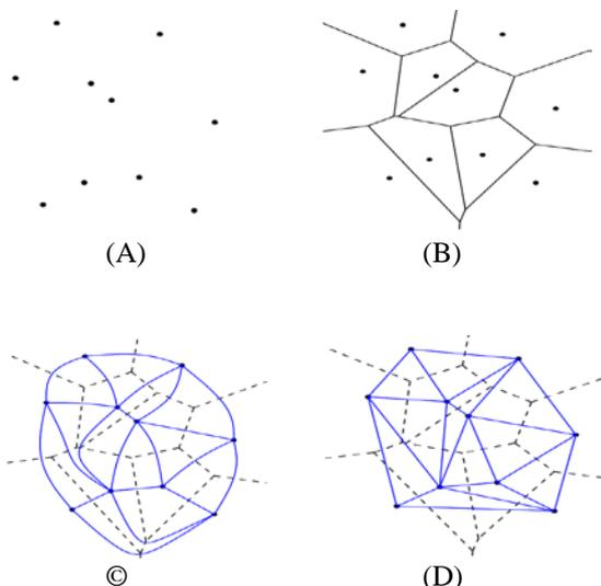
**Figure 2:** (A) Here P be the set and it has n number of point in the plane, (B) This figure is denoted it is a voronoi diagram and it subdivided of the plane into voronoi cells, (C) This one is the dual graph of voronoi diagram, (D) This is the Delaunay graph which is embedding straight line of dual graph.
