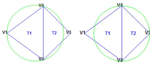
**Delaunay graph:** Delaunay Graph [65] of a set of points P is the dual graph of the Voronoi diagram of P. The Voronoi diagram  $Vor(P)$  is the subdivision of the plane into Voronoi cells  $V(p)$  for all  $p \in P$ .
