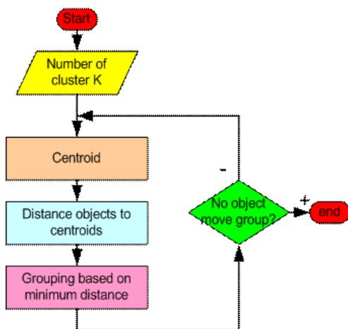
Figure 1: Flow Chart of k-means Algorithm
