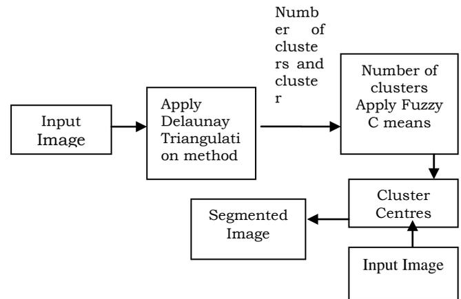
**Figure 2:** Flow chart of Delaunay Triangulation
