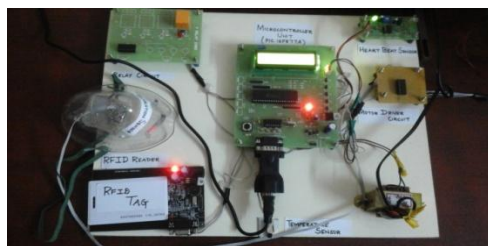
Figure 4.8. Microcontroller Unit Interfaced With Sensors, RFID.
