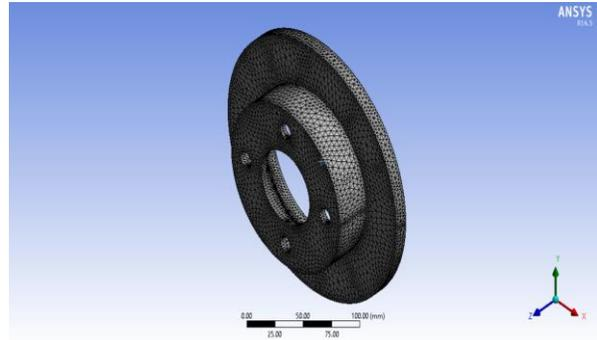
Figure 2: Meshing of the brake disc rotor
