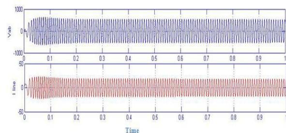
**Fig 7: Line voltage and line current of PMSG**
