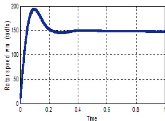
**Fig 5: Rotor Speed of PMSG**
