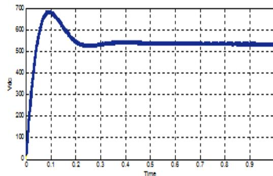
**Fig 8: DC link Voltage**
