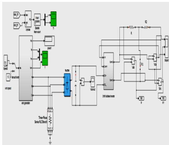
**Fig 4: Simulation model of Wind energy Conversion using CHB MLI**
