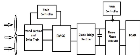
Fig 1: Block diagram of variable speed PMSG based WECS
