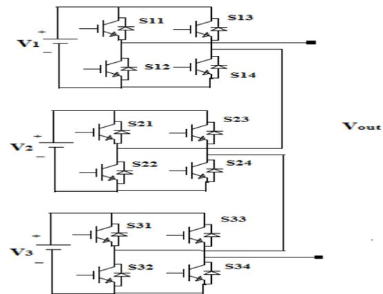
Fig 2: A Single phase cascaded H-bridge MLI
