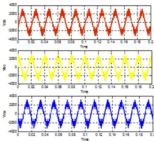
Fig 9: Line voltage of Cascaded H-bridge MLI
