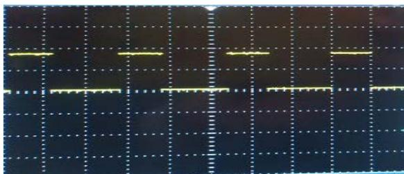
Fig.7: Gate pulse of the single MOSFET
