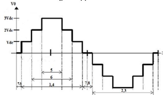
Fig.5: MOSFET switching sequence
