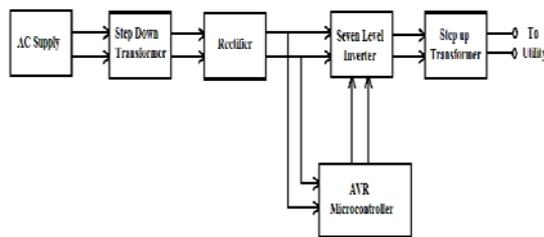
Figure 1. Block Diagram of 7 Level Inverter for power generation system
