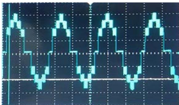
Fig.8: Output levels of the seven level inverter
