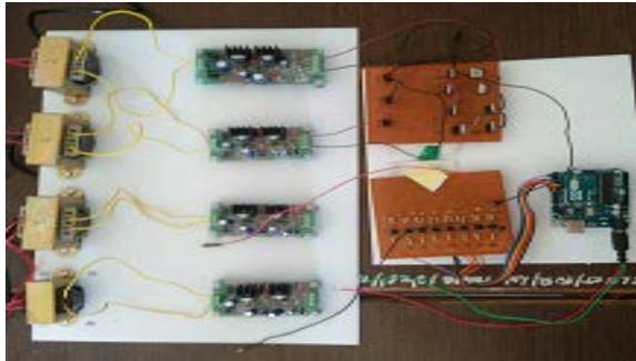
Figure 6. Actual hardware circuit of seven level inverter
