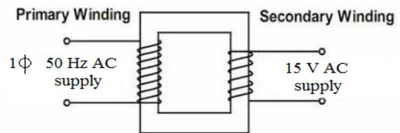
Figure 2. Step down transformer
