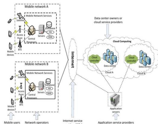
Figure: Mobile Cloud Computing Architecture
