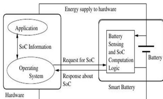
Figure: Relationship between a smartphone battery and an application.
