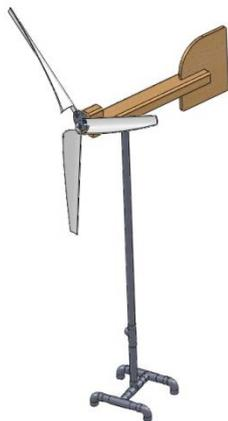
**Figure-2: Horizontal Axis Wind Turbine**
