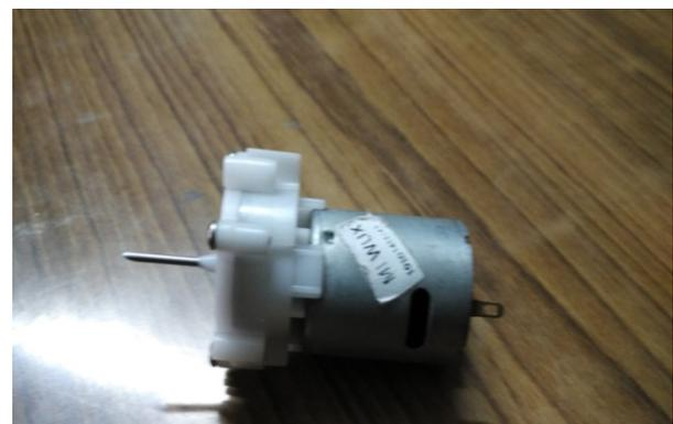
**Figure-4: D.C Motor with Pump**
