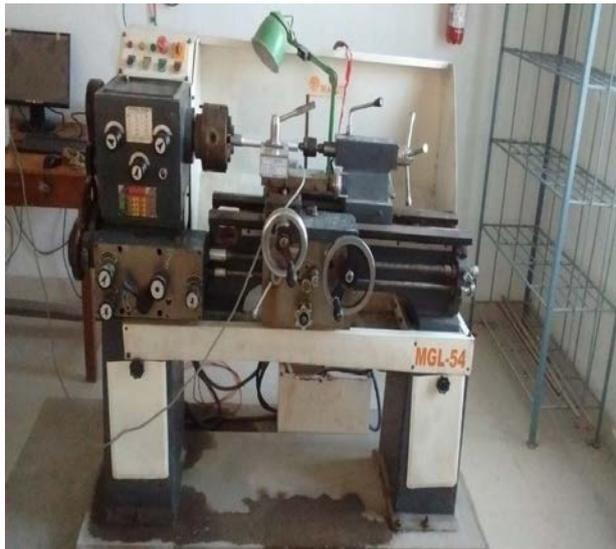
Fig 1: High Speed Lathe Machine
