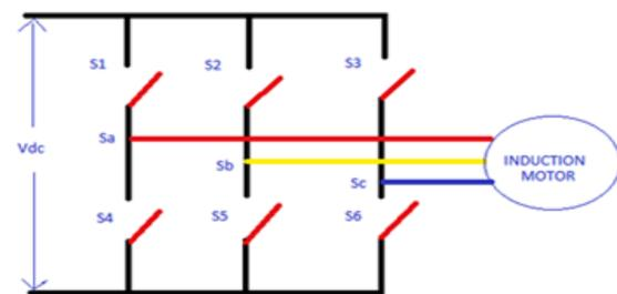
Fig.2. Schematic diagram of voltage source inverter(VSI).
