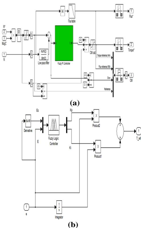
Fig.7. (a) Simulation subsystem diagram of fuzzy logic speed controller block (b) Fuzzy logic controller simulation subsystem
