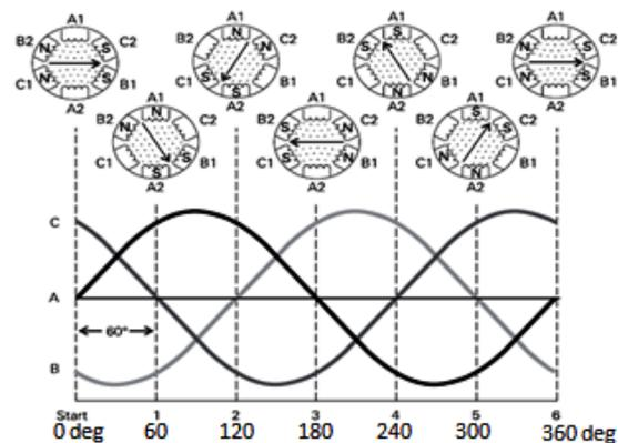
Fig.4. Rotating Magnetic Field (RMF)
