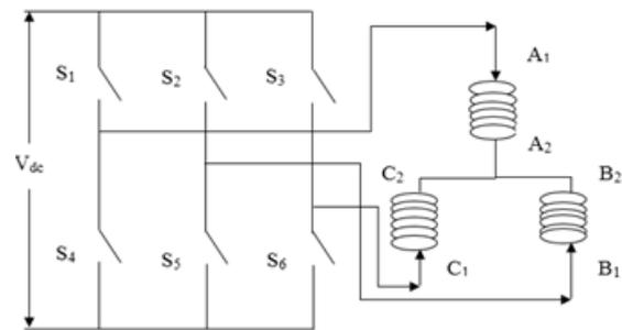
Fig.3.Three phase stator winding with VSI
