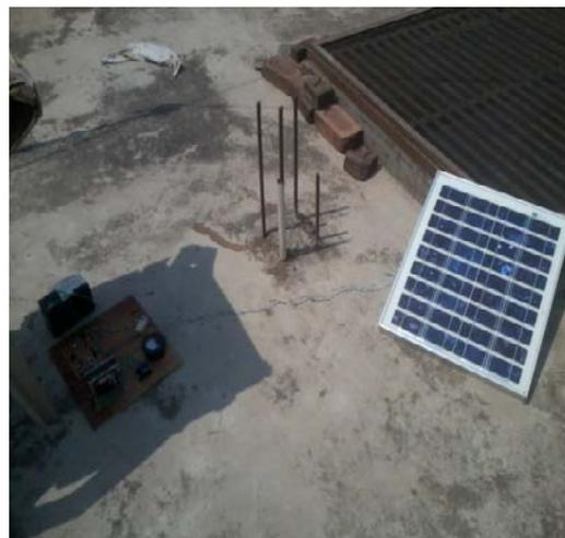
Figure 1. 20 W Photovoltaic module
