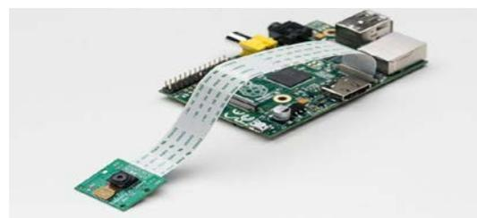
Fig.5 CAMERA INTERFACING ON RASPBERRY PI MODUL
