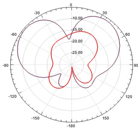
Fig.3. 2-D Radiation pattern at 3.4GHz
