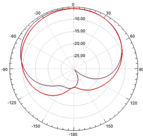
Fig.4.2-D Radiation pattern at 2.4GHz
