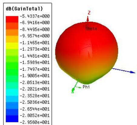
Fig.5. 3-D polar plot (gain)
