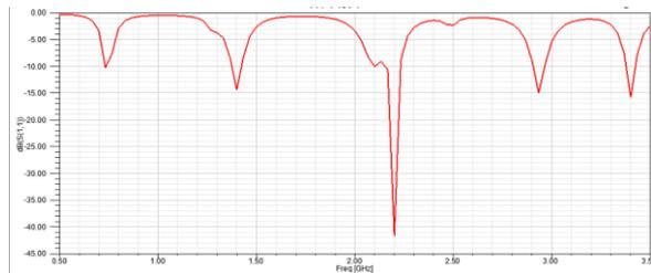
Fig.2 Reflection coefficient vs. Frequency
