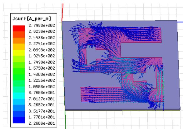
Fig.6.Surface current distribution at 2.4 GHz
