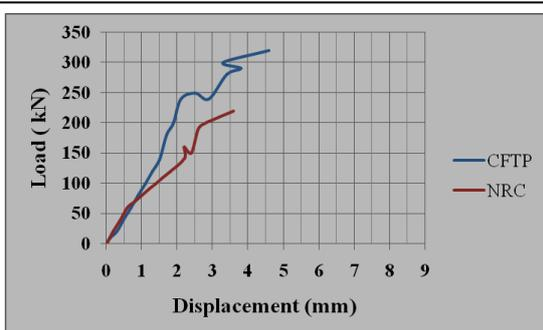
Graph 3: Load deformation curve for CFTP and RC column
