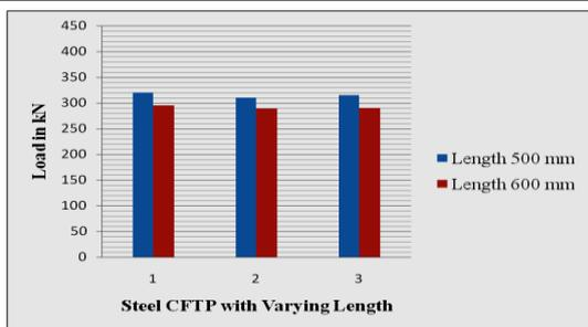
Graph 1: Load carrying capacity with length variation of CFTP
