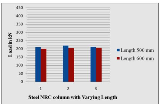
Graph 2: Load carrying capacity with length variation of RC column
