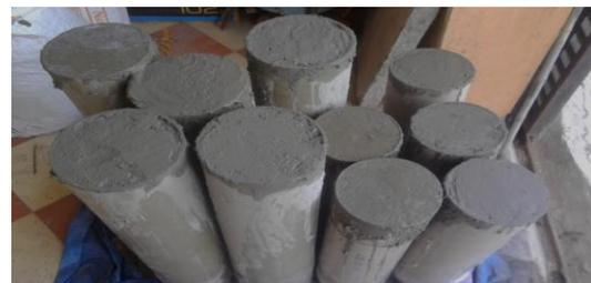
Photograph 2 Casted CFTP Specimens
