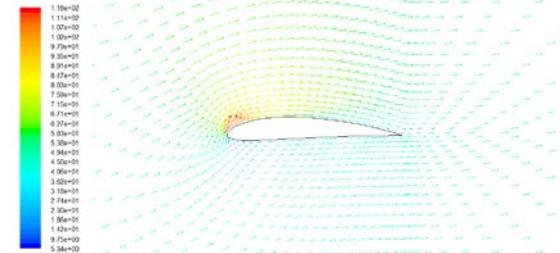
Fig.12 Velocity vector for an angle of attack 15°
