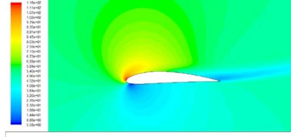
Fig.15 velocity contour for an angle of attack 15°
