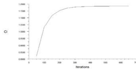
Fig.5 Plot between the coefficient of lift and number of iterations at an angle of attack 6<sup>0</sup>
