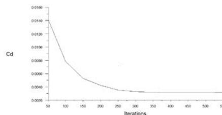
Fig.7 Plot between the coefficient of drag and number of iteration at an angle of attack 1<sup>0</sup>
