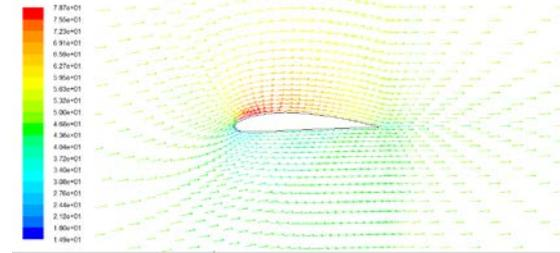
Fig.11 Velocity vector for an angle of attack 6°
