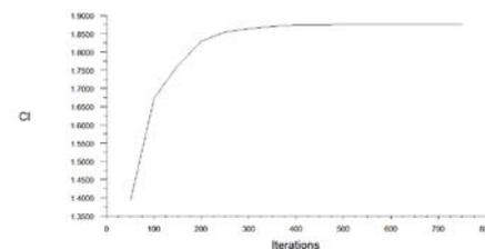
Fig.6 Plot between the coefficient of lift and number of iterations at an angle of attack 15<sup>0</sup>
