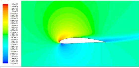
Fig.13 velocity contour for an angle of attack 1°
