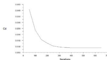
Fig.8 Plot between the coefficient of drag and number of iterations at an angle of attack 6<sup>0</sup>
