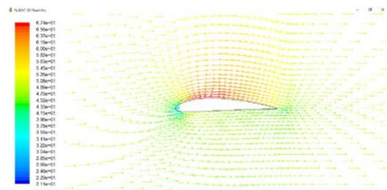
Fig.10 Velocity vector for an angle of attack 1°
