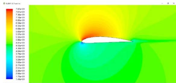
Fig.14 velocity contour for an angle of attack 6°
