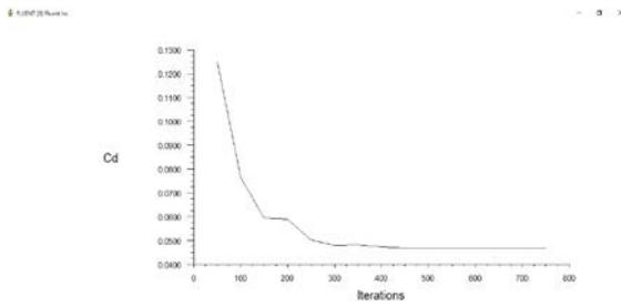
Fig.9 Plot between the coefficient of drag and number of iterations at an angle of attack 15°
