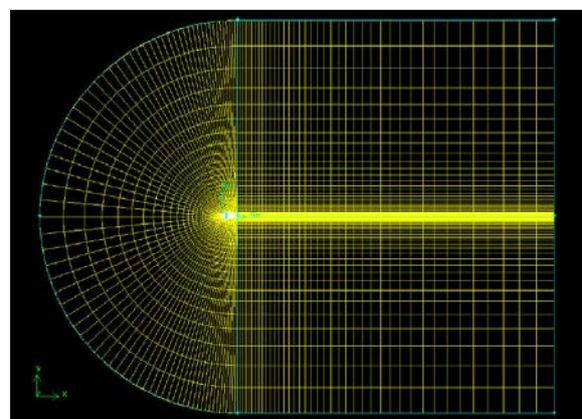
Fig.3: Final meshed region surrounding the aerofoil geometry
