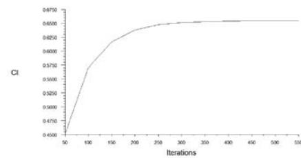
Fig.4 Plot between the coefficient of lift and number of iteration at an angle of attack 1<sup>0</sup>
