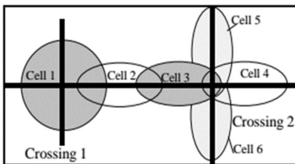
Figure 4 : Network topology with two cellular patterns for crossings. (Source: Dialog Telecom)
