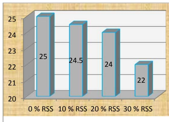
**Graph: 1 Representation of Slump Cone Test**
