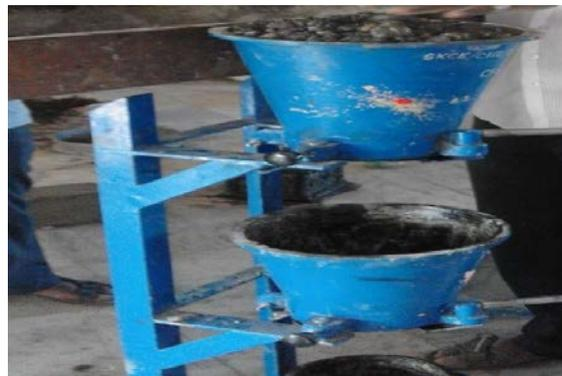
**Fig: 4 Compaction Factor**
