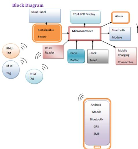
Fig1: Block Diagram Of Smart Bag
