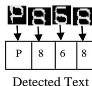
The obtained text is compared with the database and if the text matches a signal is sent to the board which activates the mechanical motion i.e., opening of the gate. If the text does not match it alerts the security by providing a buzzer sound for security purpose.
