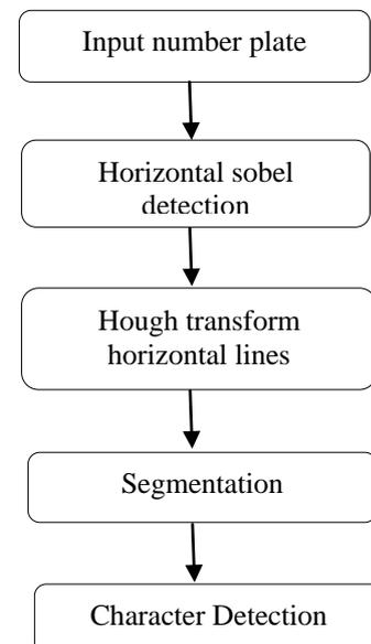
The information from the input image is first processed using Sobel edge detection which detects all the edges present in the image and then Hough transform is applied for the detection of horizontal lines present in the images. After the successful detection using Hough transform, the letters present in the image is segmented by finding the end points in the characters.
