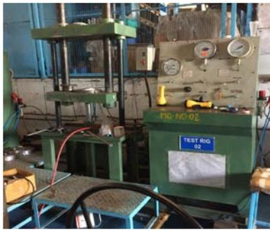
Figure No.1 Existing test rig for ball valves.
