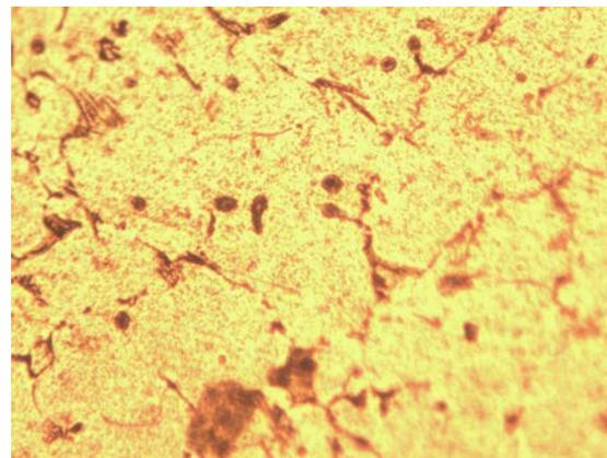
**Fig 2: Microstructure of Al-CSAp composite**
