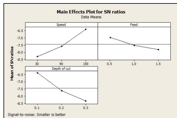
**Fig 4: main effect plot for S/N ratio for aluminium**
