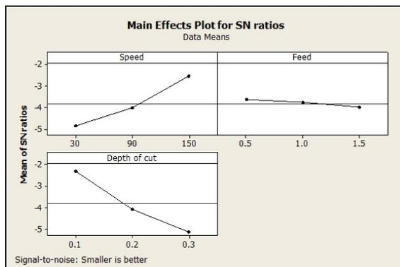
**Fig 5: main effects plot for SN ratio for Al-CSAp**
