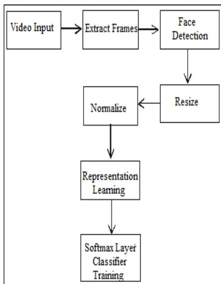
Figure 3. Algorithm Face Detection
