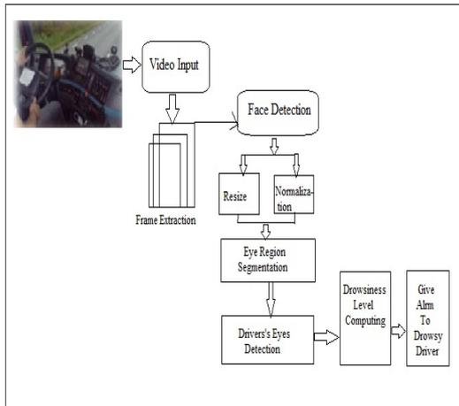
Figure 2. System Architecture
