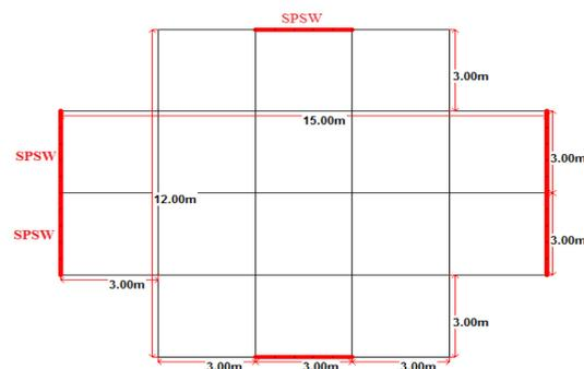
**Fig -3: Plan of a steel frame building with steel plate shear wall**
