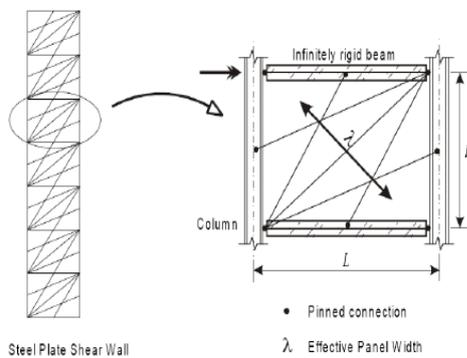
**Fig -2: Multi-angle strip model of a SPSW**
