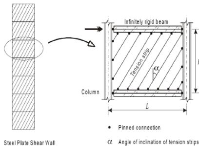
**Fig -1: Strip Model Representation of a SPSW**
