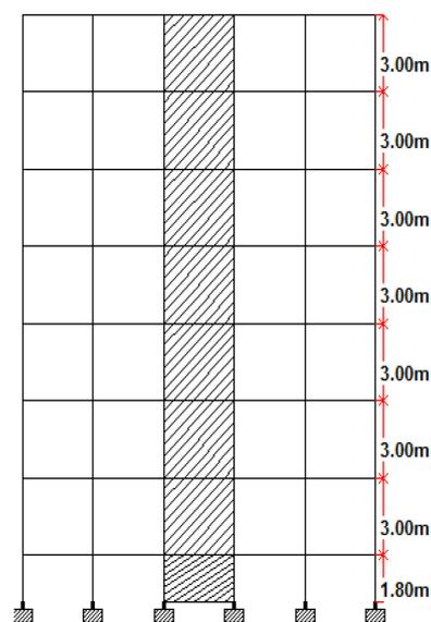
**Fig 4: Elevation of a steel frame building with steel plate shear wall**
