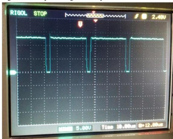
Figure 15: Off state voltage waveform (Vds) across the switch
