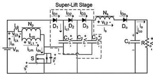
Figure 1: Circuit diagram of the converter
