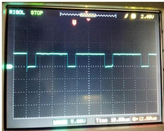
Figure 13: Plot of duty ratio obtained across CRO
