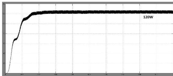
Figure 11: Output power plot at 1200W/m<sup>2</sup>
