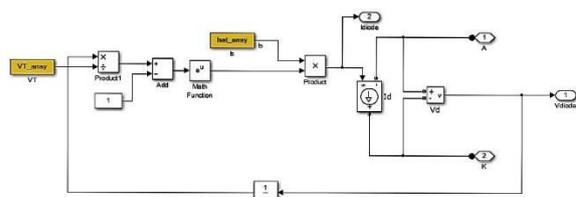
Figure 4: The diode model used in the solar array
