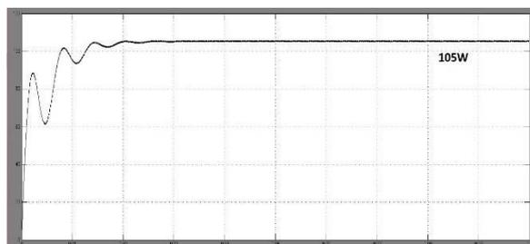
Figure 7: Input power v/s time plot without MPPT
