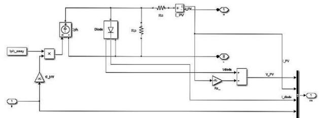
Figure 2: Kyocera 135GX-LP panel's solar array model. By varying the irradiance level, we can extract V v/s I and P v/s V graph to find MPP of solar array shown in fig 3.
