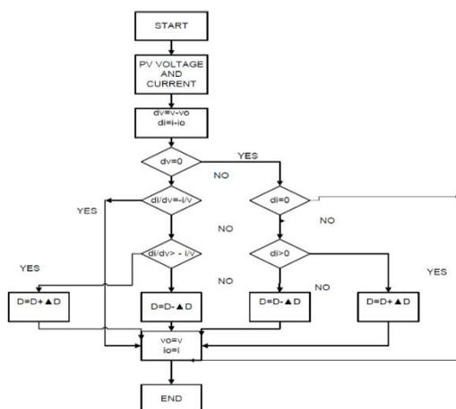
The flow chart for INC algorithm is shown in fig 5.
