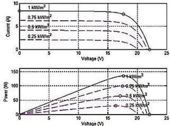
Figure 3: P v/s V and I v/s V plot for the solar array modelled
