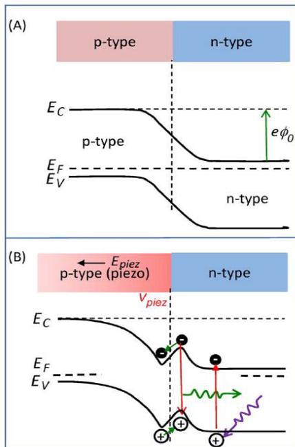
Fig.2. Energy band diagram for illustrating the effect of piezoelectricity on a pn junction. (A) Band diagram at a conventional pn junction made by two semiconductors have almost the same bandgaps. (B) Band diagram of the pn junction with the presence of a piezopotential at the p-type side with a polarity of higher potential at the junction side.
