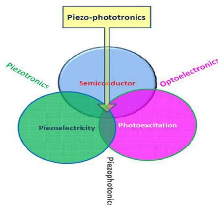
Fig.3. Schematic diagram showing the three-way coupling among piezoelectricity, photoexcitation and semiconductor, which is the basis of piezotronics (piezoelectricity—semiconductor coupling), piezophotonics (piezoelectric—photon excitation coupling), optoelectronics, and piezo-phototronics (piezoelectricity—semiconductor—photoexcitation). The core of these coupling relies on the piezopotential created by the piezoelectric materials.
