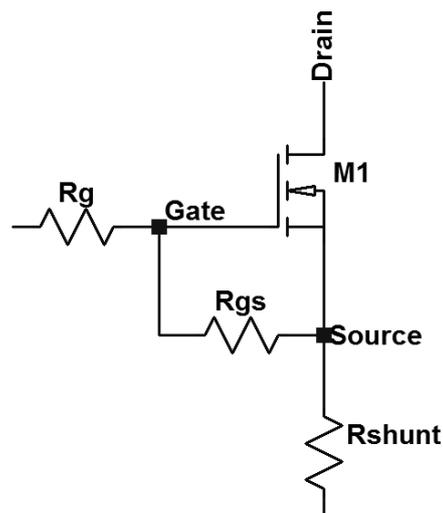
Figure 3. Equal current sharing requirements.
