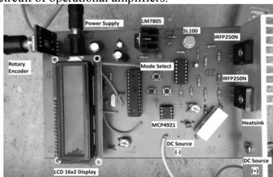
Figure 6. The electronic load hardware.
