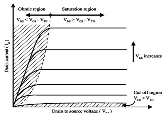
Figure 1. Characteristics of a power MOSFET [3].
