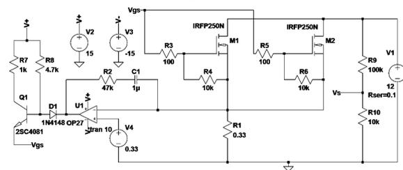
Figure 5. The electronic load set-up.
