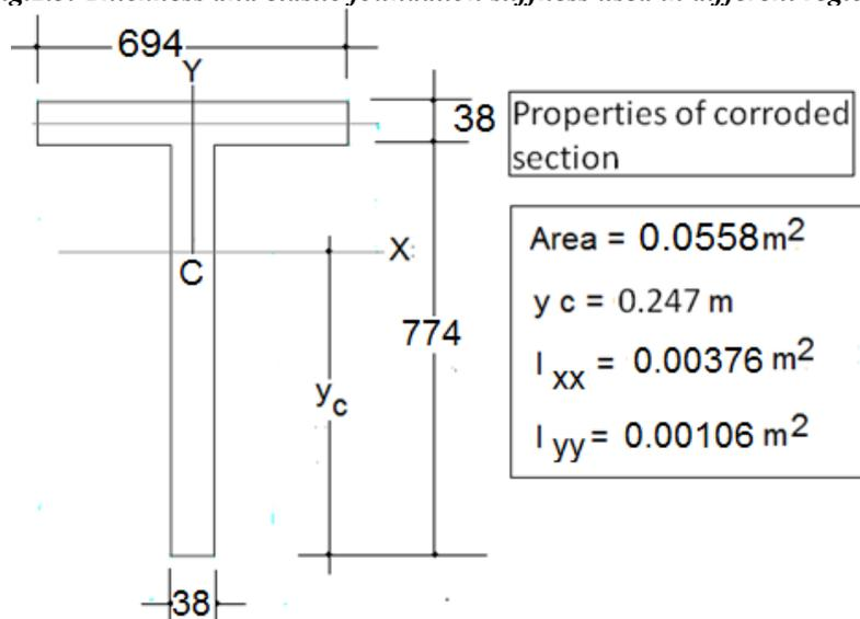
Fig.2.4. The cross-section of the stiffener
