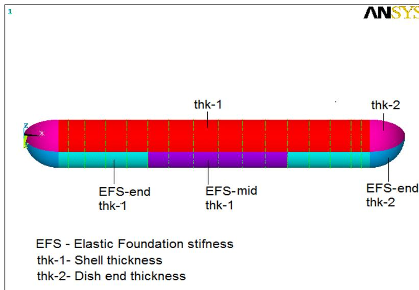
Fig.2.3. Thickness and elastic foundation stiffness used in different regions.
