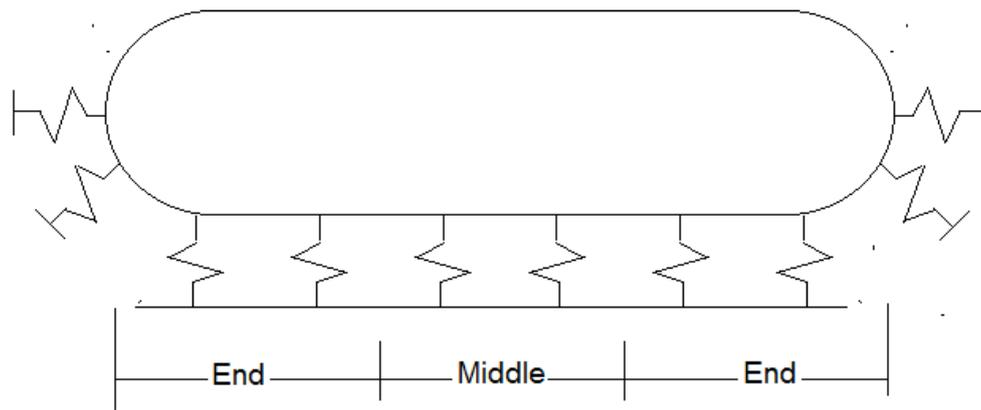
Fig.2.5. Vessel on elastic foundation
