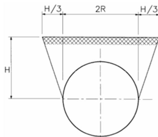
Fig.2.6. weight of mound on the vessel
