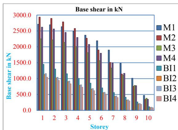
Figure 11. Comparison of Base shear of fixed models and base isolated models in kN.
