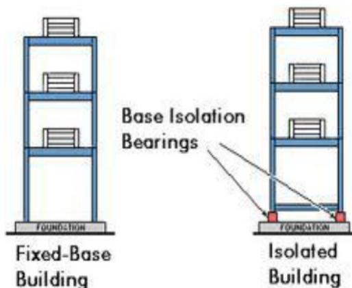
Figure 2. Function of base isolation.
