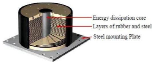
**Figure 4. Lead rubber bearing.**
