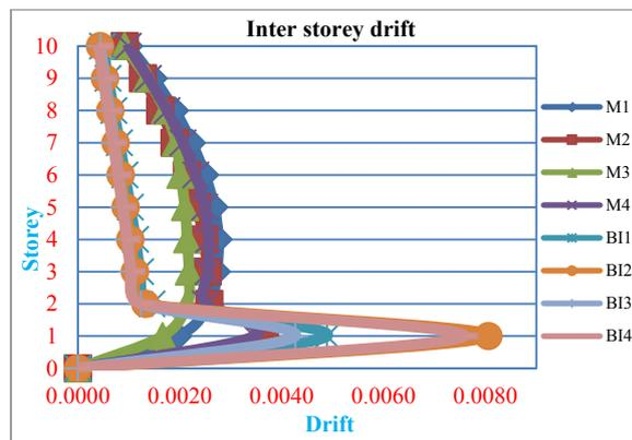
Figure 10. Comparison of Inter storey drifts of fixed models and base isolated models.
