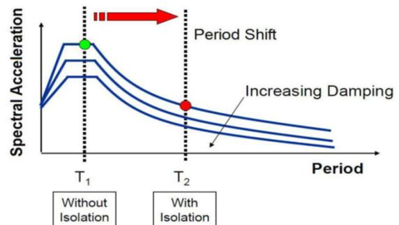
Figure 3. Period shift effect of fixed base and base isolated building.
