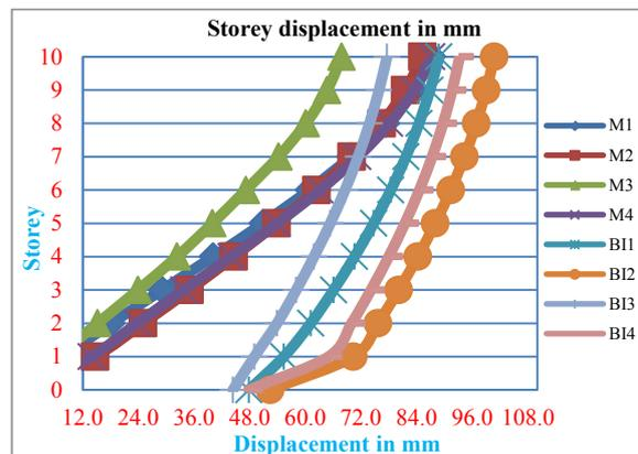
Figure 9. Comparison of lateral displacement of fixed models and base isolated models in mm.
