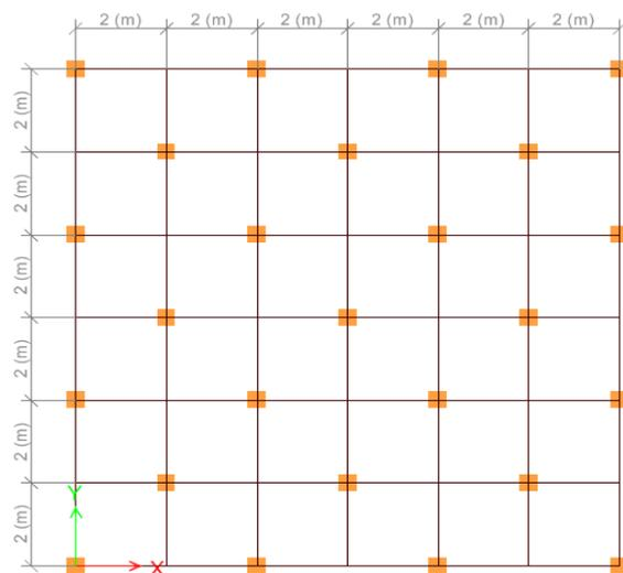
**Figure 5. Regular building with floating column (M2).**
