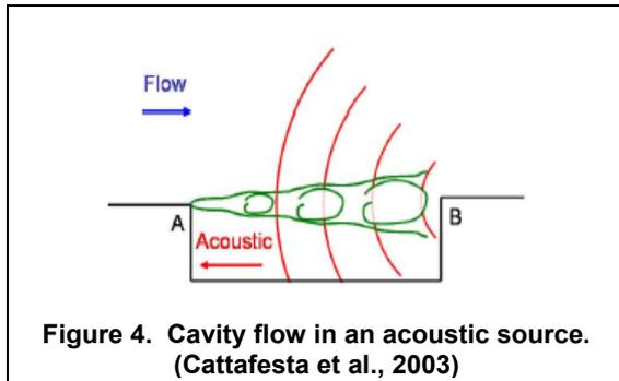
Figure 4. Cavity flow in an acoustic source. (Cattafesta et al., 2003)
