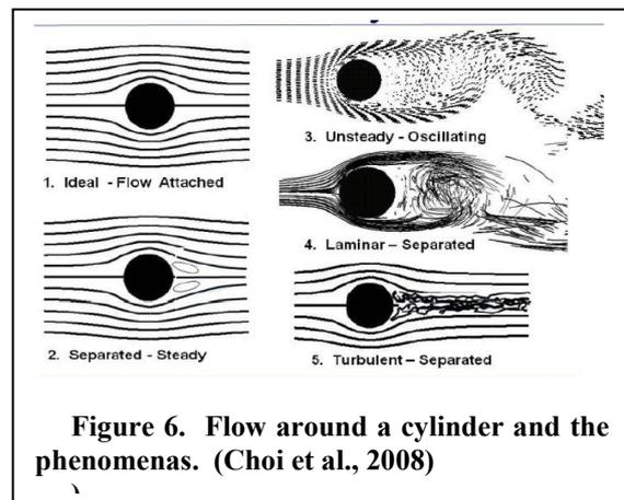
Figure 6. Flow around a cylinder and the phenomena. (Choi et al., 2008)
