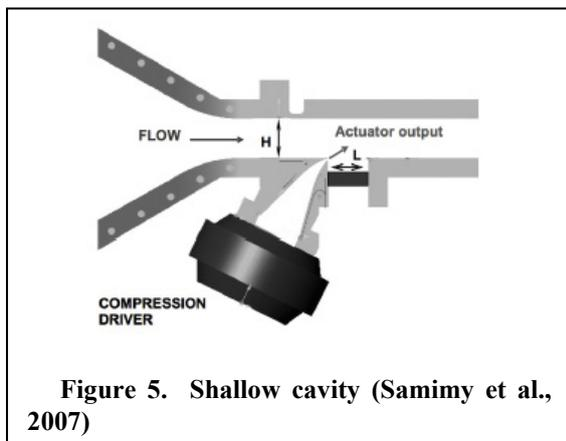
Figure 5. Shallow cavity (Samimy et al., 2007)
