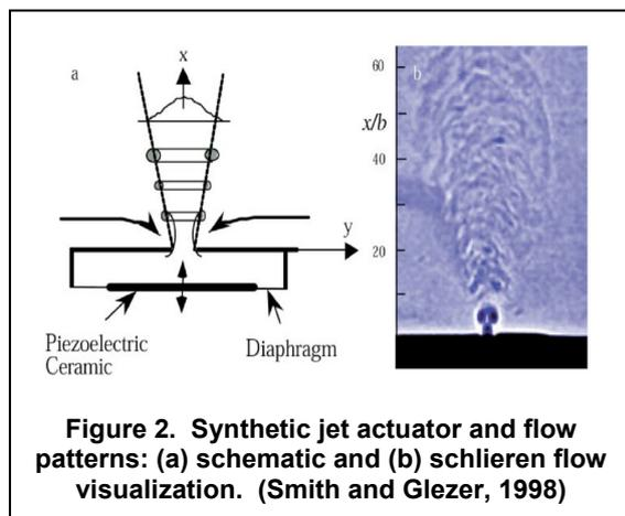
The use of actuator to control flow is typically accomplished through a wide variety of processes like; virtual surface shaping, thrust-vectoring, separation control and mixing enhancement (Amitay et al., 2001).
