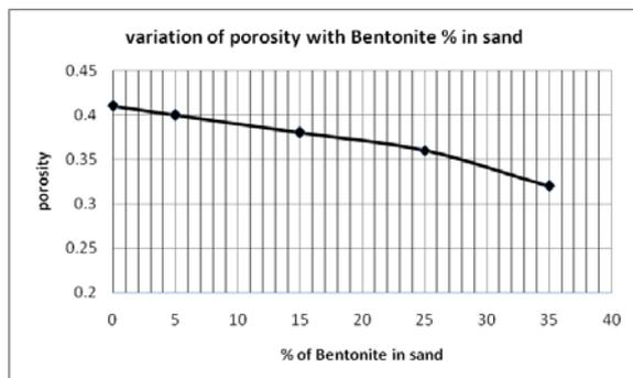
Figure 4 plot between porosity and % of Bentonite in sand
