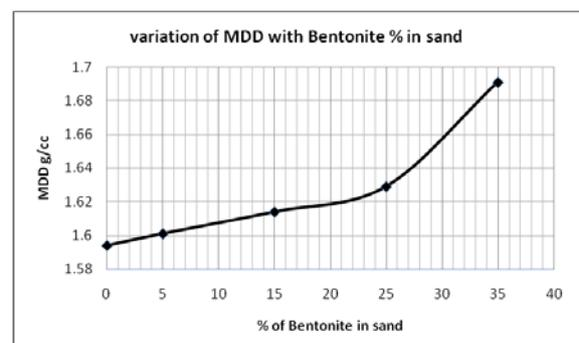
Figure 2 plot between MDD and % of Bentonite in sand
