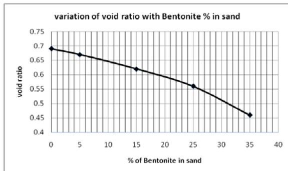
Figure 3 plot between void ratio and % of Bentonite in sand
