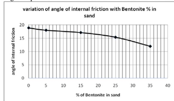
Figure 6 plot between angle of internal friction and % of Bentonite in sand
