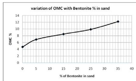
Figure 1 plot between OMC and % of Bentonite in sand
