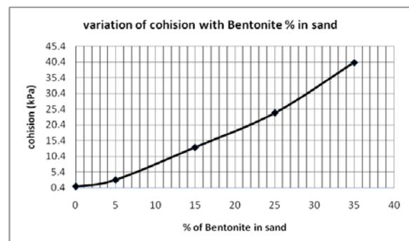
Figure 5 plot between cohesion and % of Bentonite in sand
