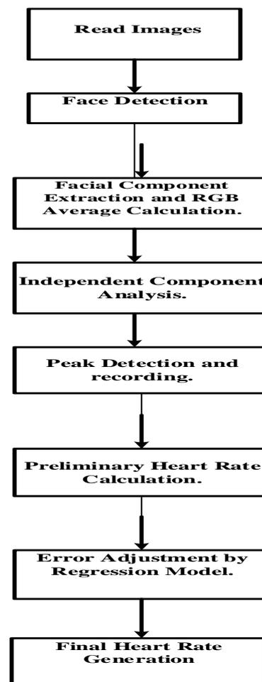
Fig. 1. Overall system flow showing processes running on the user end and on the server.
