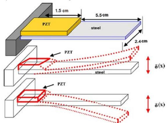
Fig.2 1. A 3D view of the experiment setup
