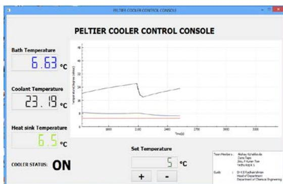
Figure 6- Maximum cooling test results on GUI
