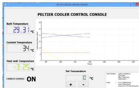
Figure 8 - Free convection test result on GUI
